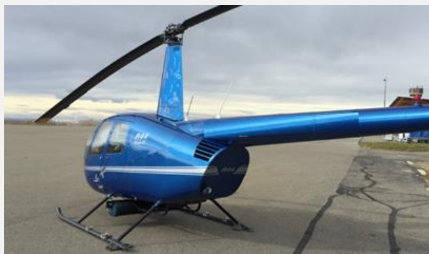
Measurement Cell mounted on a Robinson R44
