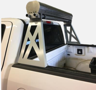
GasFinder3-VB on Headache Rack Mounting Structure
